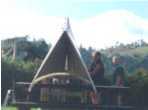
Two hull panels with sheer line spread to deck width.
