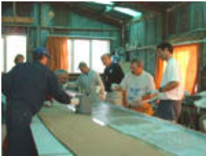
Applying the inside skin to a hull panel on the first day.
