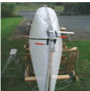
After shaping. Note the steel 'T-piece' along centre line.
