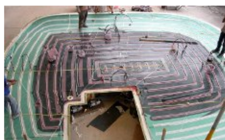
KSS 58's Saloon top (7m x 6.5m) being resin infused, in one shot, in Peru
