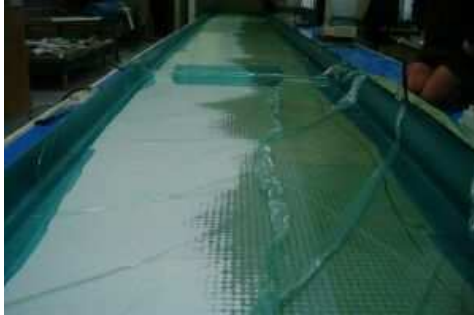
70' top side panel – 10 minutes into resin infusion
