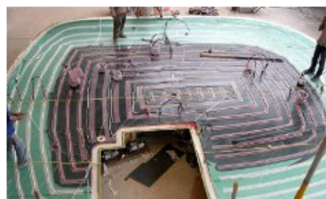
KSS 58's Saloon top (7m x 6.5m) being resin infused, in one shot, in Peru
